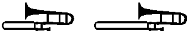
The natural frequency of a trombone can be modified by changing the length of the air column inside the metal tube.
