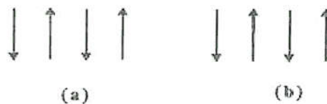
Fig. 5.4 Relative orientation of electron spins in (a) antiferromagnetic material and (b) ferrite.
